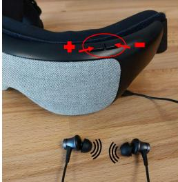
To adjust the sound level, use the buttons on the top of the device. You will find them with your **left hand** when you are wearing the device.
